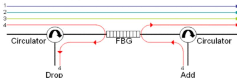
Fig.5.2 optical add- drop multiplexing
