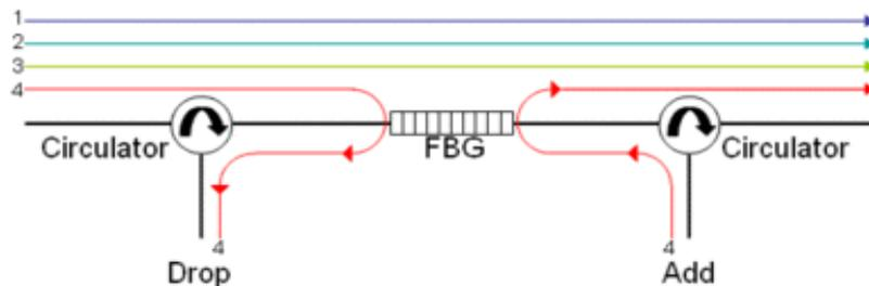
Fig.5.2 optical add- drop multiplexing
