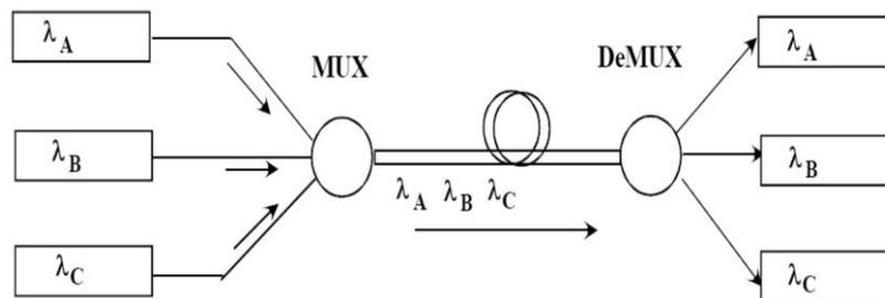
Fig 5.1 wavelength division multiplexing
